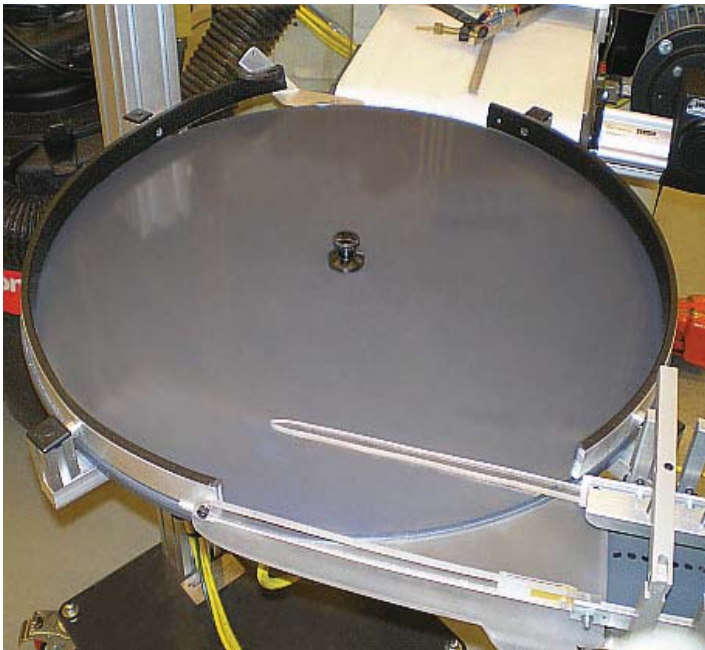
ACTUAL APPLICATION: Fixed-Fence option with custom suspended exit rail system; table modified with non-standard gearmotor for high-speed 90-degree product transfer.
