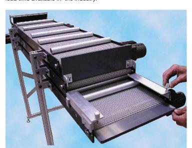
ACTUAL APPLICATION: Three 16" by 60" Lite modules in custom triplestack decline mounting, for overnight parts collection in a 1-1/2-foot by 5foot area of available floor space. Included custom cycle timer and custom parts delivery system, with raised-surface rubber belting and pneumatic actuated parts stop. 2.5 weeks delivery turnaround ARO.
