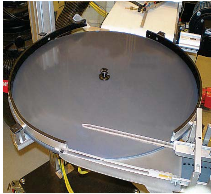
ACTUAL APPLICATION: Stationary Fence option with custom suspended exit rail system; table modified with non-standard gearmotor for high-speed 90-degree product transfer.
