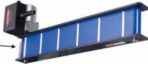
Fig. 14 Install discharge ramp on conveyor
