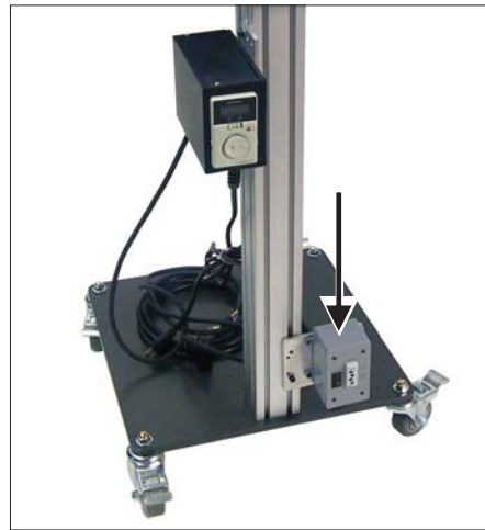
Fig. 7a Allow the timer to slide out of the way until later adjustment.
